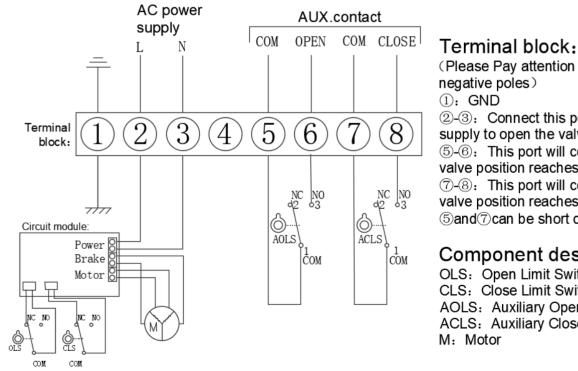
(Please Pay attention to the positive and negative poles) (1): GND 2-3: Connect this port with AC power supply to open the valve 5-6: This port will connect when the valve position reaches full Close; 7-8: This port will connect when the
