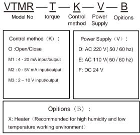
The M2 and M3 control methods need to be developed, and if this control is chosen, the delivery time will be delayed \*The above information is for reference only. If you are interested, please consult the factory in advance
